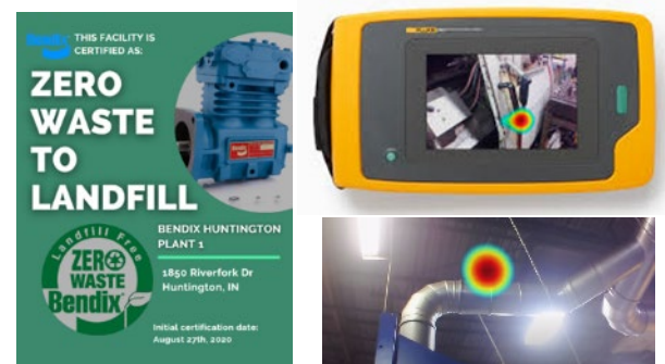
Above: (Left) Bendix Huntington Plant Zero Waste to Landfill Certification; (Top and Bottom Right) Fluke ii900 Sonic Industrial Imaging camera used to detect leaks.
